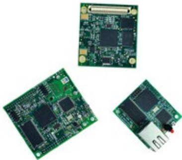
**SYNC 200** are embedded system on module (SOM) boards which can be directly plugged into field equipment/ devices to enable it with multiple protocols without changing the core hardware.
